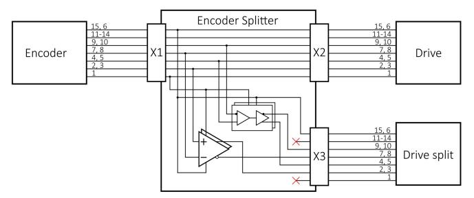
Figure 2: Schematic of the wiring inside the TAES encoder splitter.
