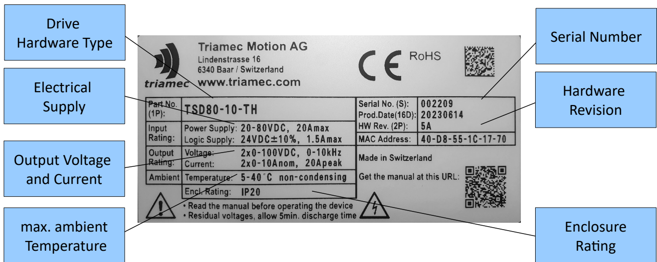
Figure 1: Nameplate of the TSD series servo drives
