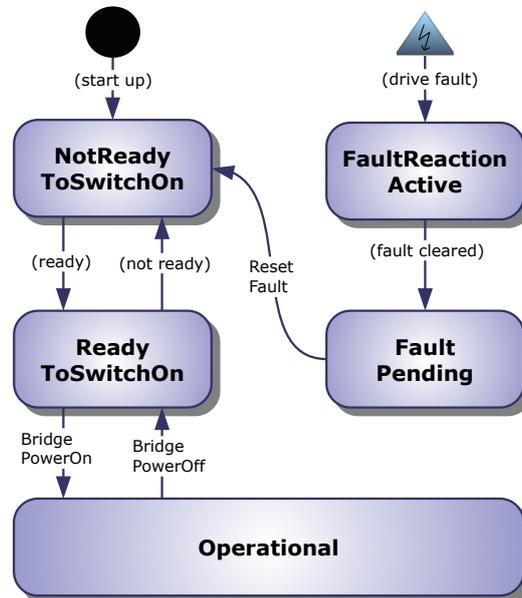
Figure 11: Device State Machine
