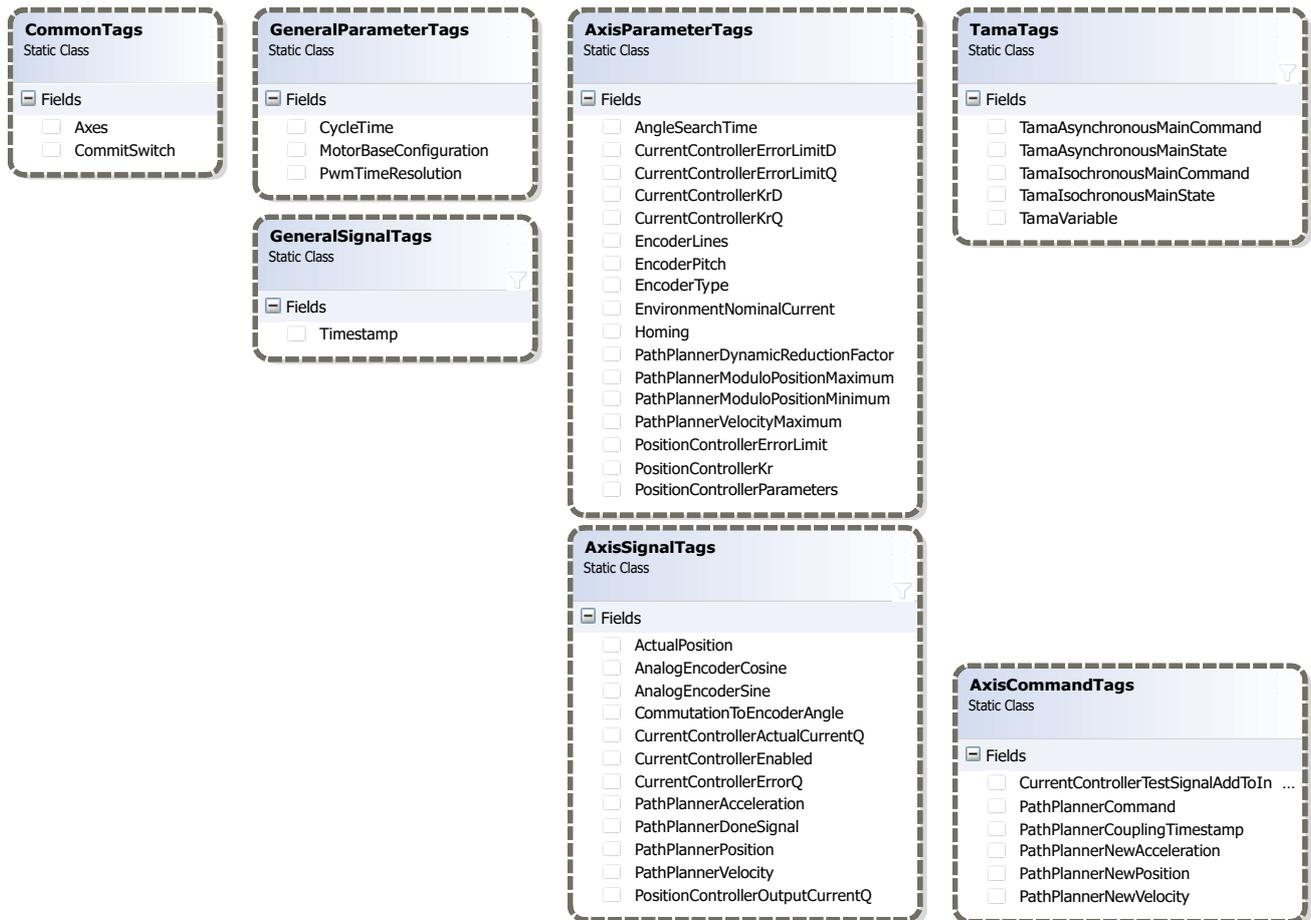
Figure 24: The most commonly used register tags
