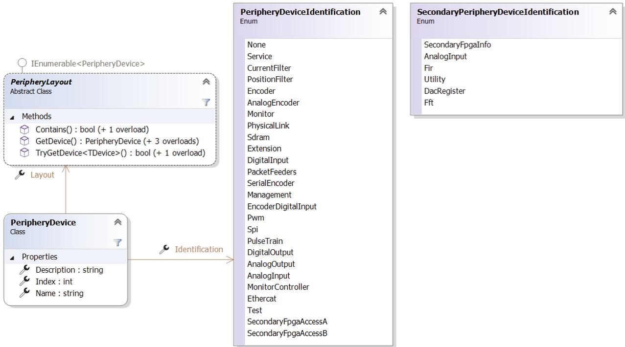
Figure 22: Get a peripheral device
