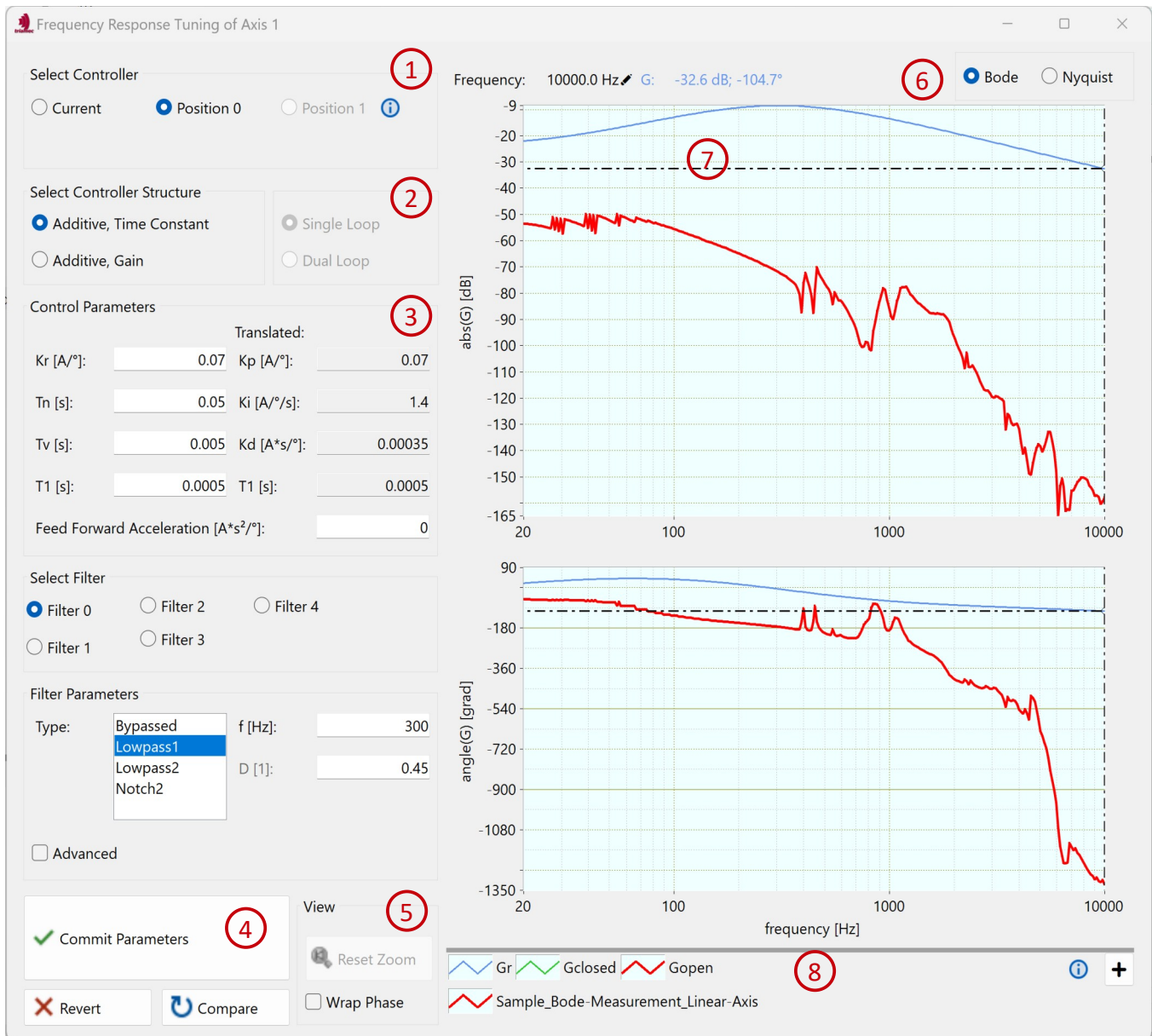
Figure 38: Frequency Response Tuning editor with current controller and Bode plot selected.
