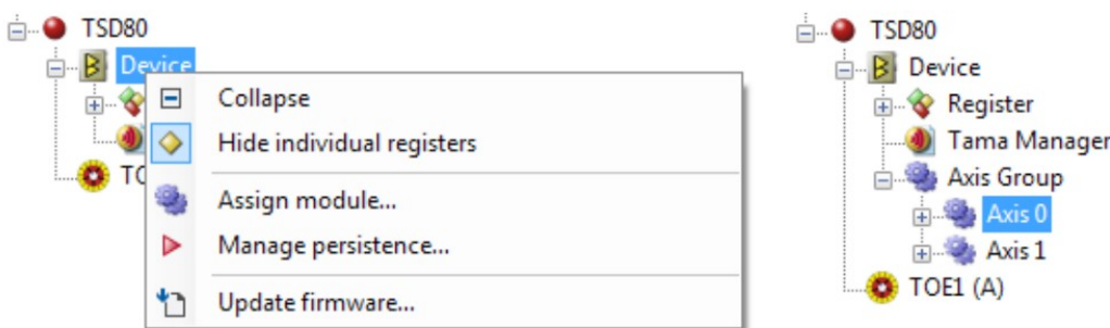
Figure 32: Axis module assignment.
