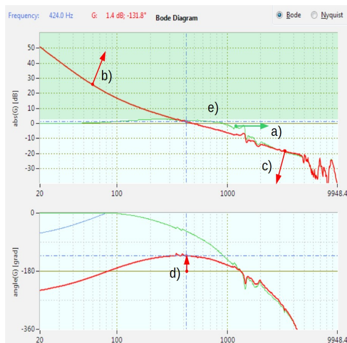
Figure 62: Tuning criteria in Bode view for the position controller.
