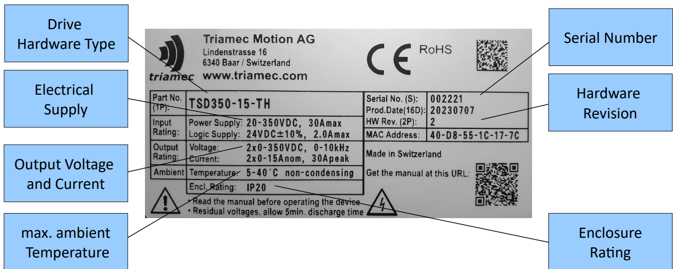
Figure 1: Nameplate of the TSD series servo drives
