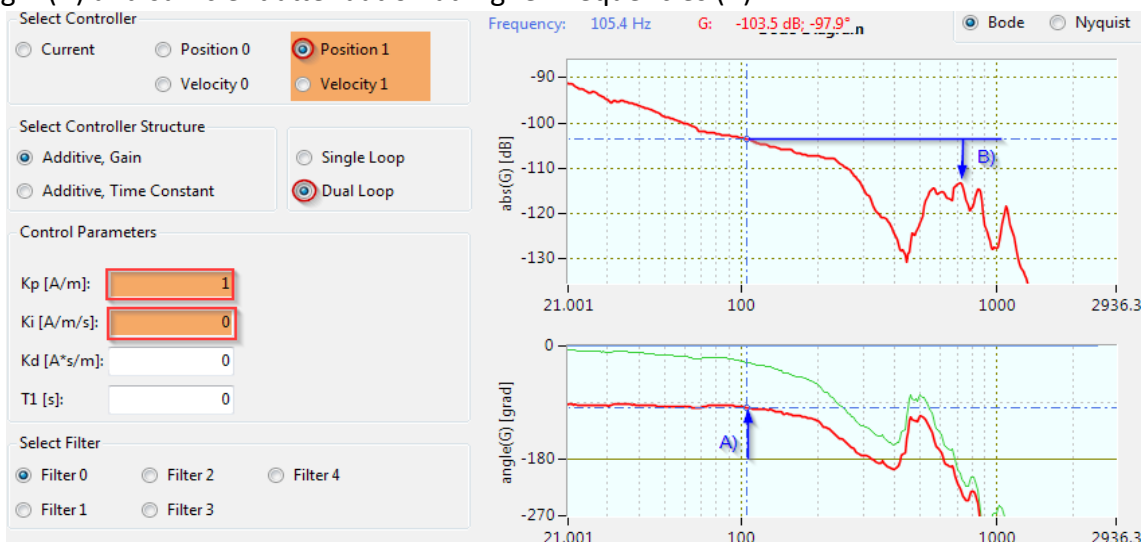
Figure 8: Tuning of outer loop: A) phase margin; B) attenuation at higher frequencies.
