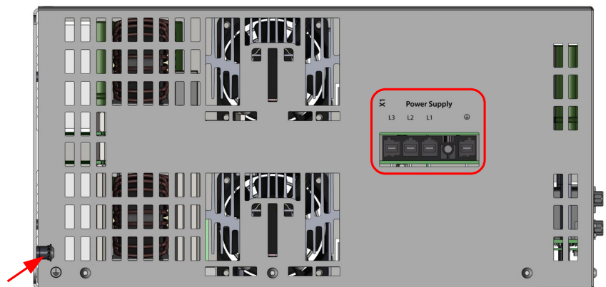
Figure 7: AC-power supply connector (X1) TSP700-40
