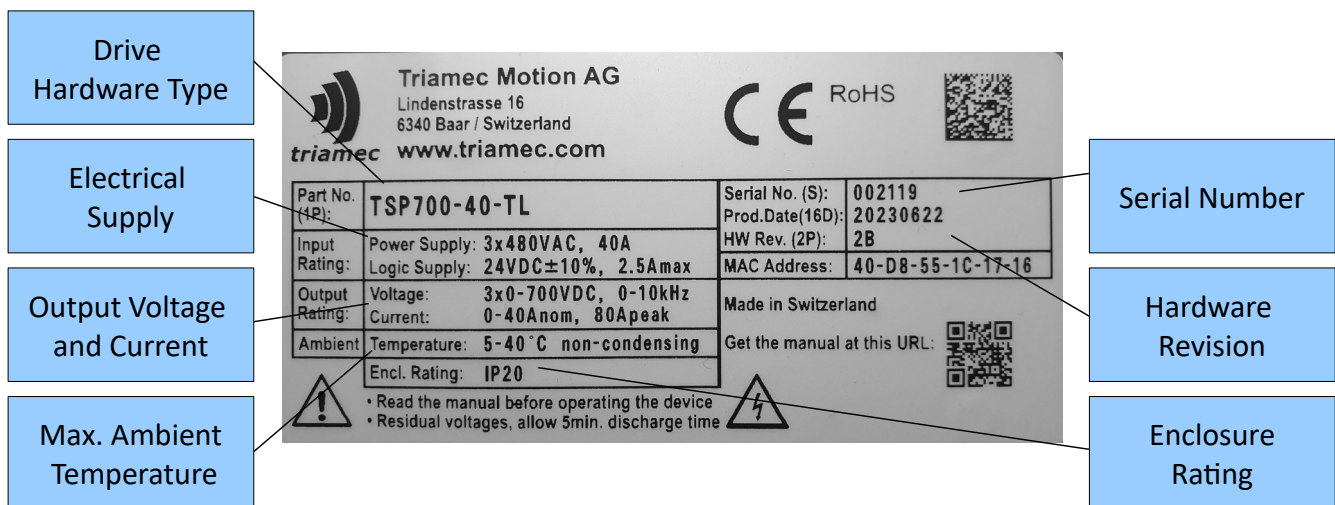
Figure 1: Nameplate of the TSP series servo drives
