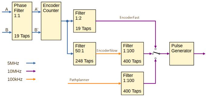
Figure 3: Signal path of the pulse position source
