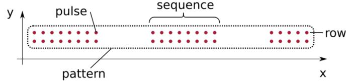
Figure 1: Visualization of Pulsing Unit specific terms
