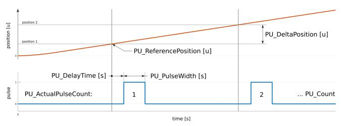
Figure 5: Visualization of Pulsing Unit parameters
